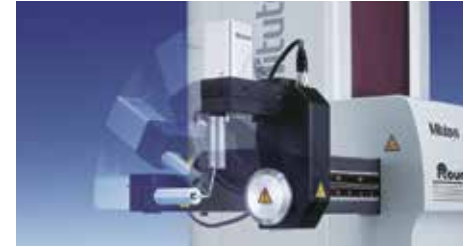
Holder-arm orientation switching (vertical position - horizontal position)
