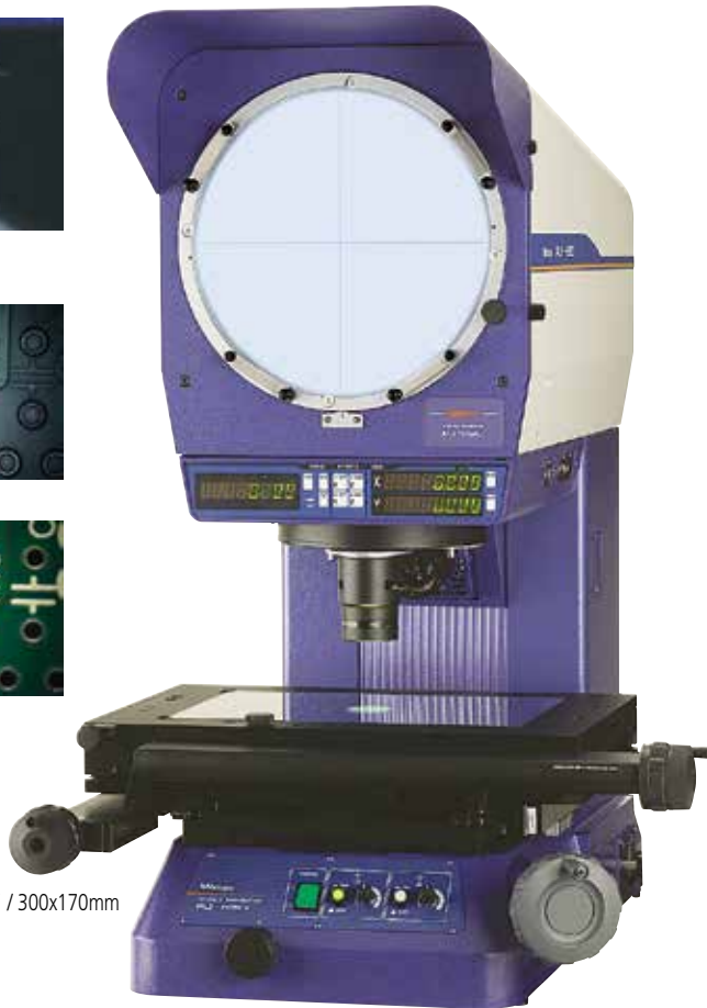
Adjustable / oblique switchable surface illumination
