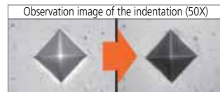
Stray light reduction around the indentation
