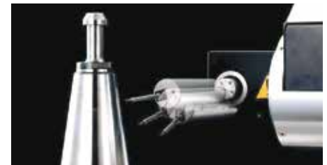
Detector rotation mechanism (0 to 290°, in increments of 1°)
