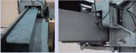
Integrated Y-Axis in Granite Table
